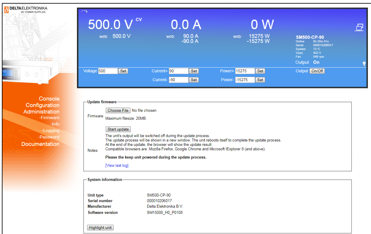
fig 7 - 3 - Via the web interface the downloaded firmware package can be uploaded to the unit.
