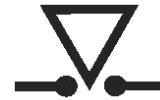
fig 6 - 11 The Interlock symbol will be visible in the display when the link is interrupted.
