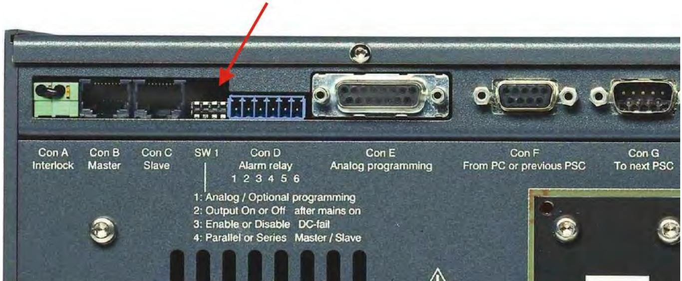
Set dip switch 5 of switch SW1 in the position 'down'. After switching mains on, the unit will always start up with a voltage setting of 0 V and a current setting of 0 A. Once the unit is switched on, the voltage and current can be set to the preferred value.
