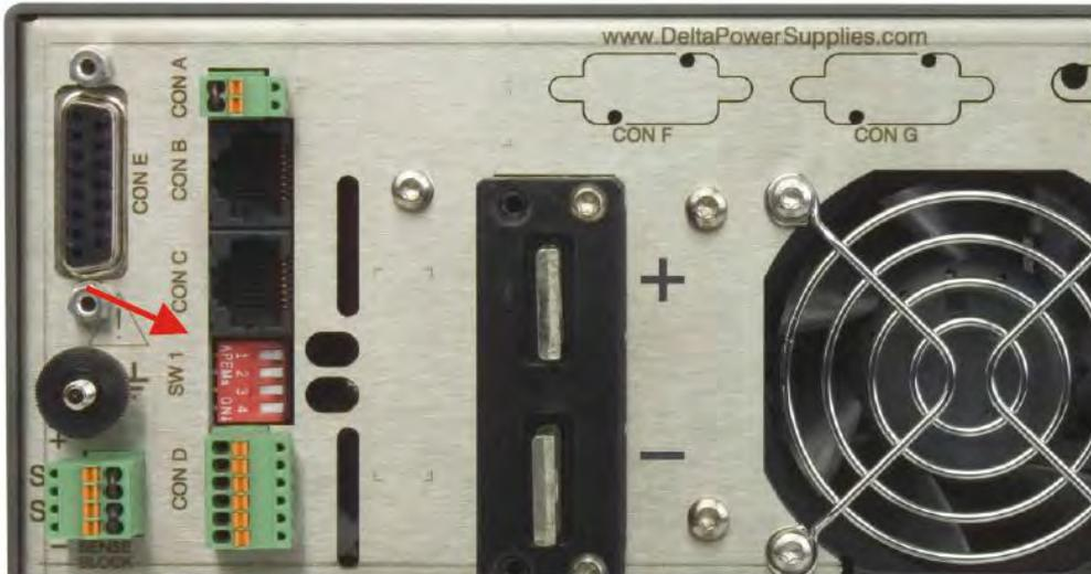
Set dip switch 5 of switch SW1 in the position 'down'. After switching mains on, the unit will always start up with a voltage setting of 0 V and a current setting of 0 A. Once the unit is switched on, the voltage and current can be set to the preferred value.
