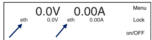
fig 6 - 18 The programming source appears before the settings. In this example both CV and CC settings are controlled via Ethernet.
