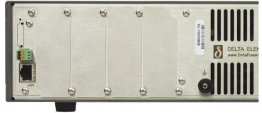
fig 8 - 3 The location of the LAN-connector and the available interface slots at the rear panel.
