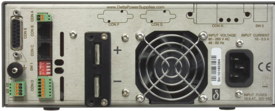
fig 4 – 8 Location of output terminals and analog programming connector on the rear panel.
