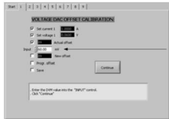
Screen 1: Voltage DAC Offset calibration
