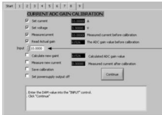
Screen 8: Current ADC gain calibration
