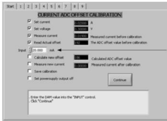
Screen 7: Current ADC offset calibration
