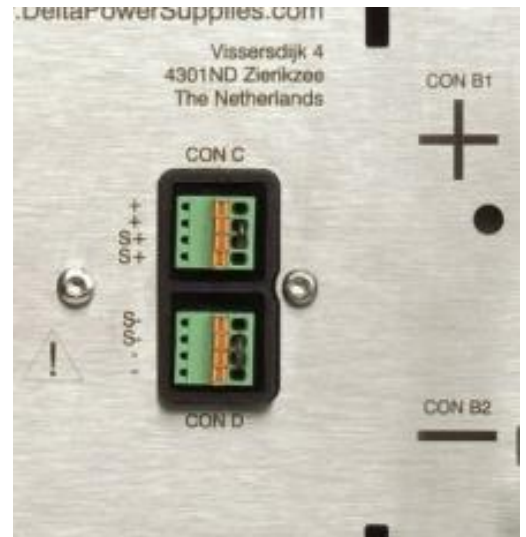
fig 9 - 2 For normal operation links should be connected between S+ and +, and between S- and -. Note that there is room for two links in each sense block but it is sufficient if one is connected.
