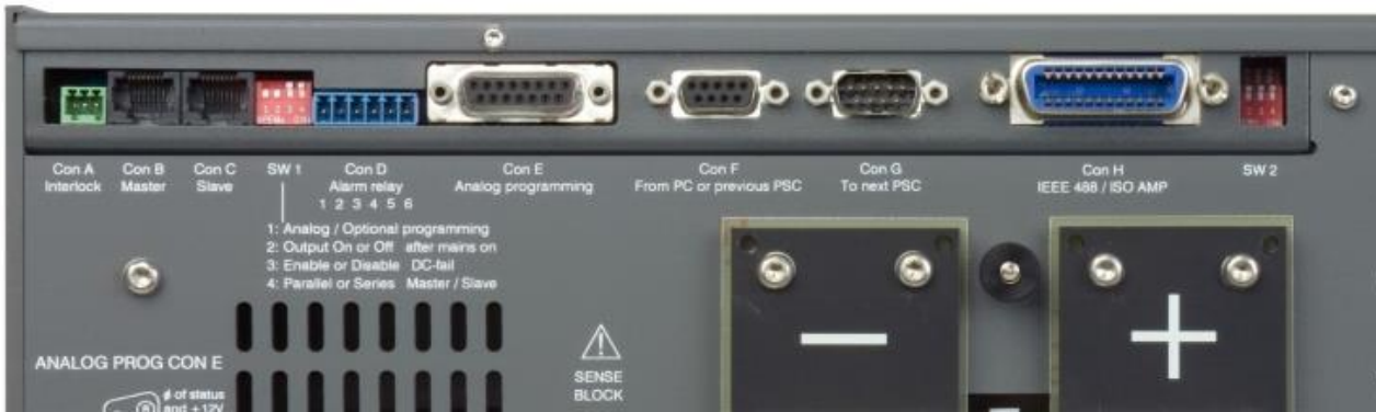
fig 4 – 8 Location of output terminals and analog programming connector on the rear panel.
